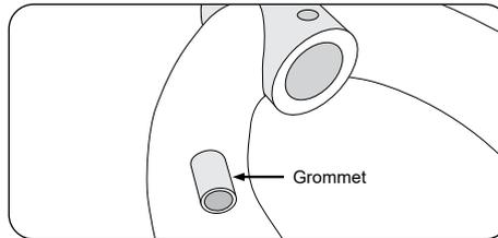
If there is no grommet, the cable must be fixed into place on the fork leg with black cable ties. Ensure that the cable is not compressed. Cut the rest of the cable ties that are sticking out. The cut end of the cable tie should be turned towards the inside of the fork.
