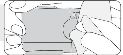
3. Mount the handlebars. Place the handlebars in the centre of the stem and position it facing backwards on the top pipe. Put the stem plate on and screw all four bolts back in clockwise. Tighten the bolts evenly and only lightly cross-wise.
