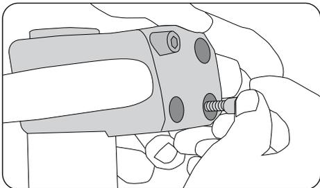
4. Straighten the handlebars. They must sit in the centre of the stem. They should be parallel to the fork when you look at the bike from the side. Screw in the bolts in the stem plate cross-wise. The correct tightening torque is **8 Nm**
