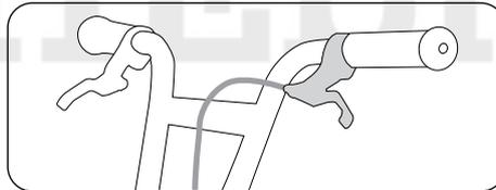
3. Orient the brake lever so that you can always apply the brake safely. The brake lever should be tilted slightly forwards and down.
