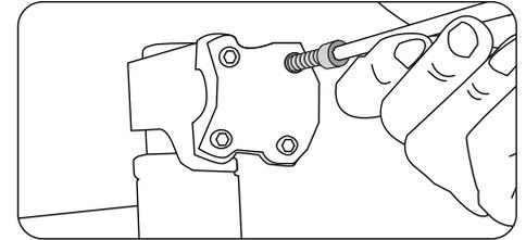
2. Carefully grease the clamp surface of the stem and handlebars.
