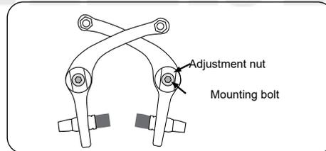
2. Tighten the adjustment nut with a suitable open-end wrench. Maximum of a quarter-turn should be enough.
