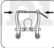
2. Loosen the cable clamp bolt until the cable can be moved.
