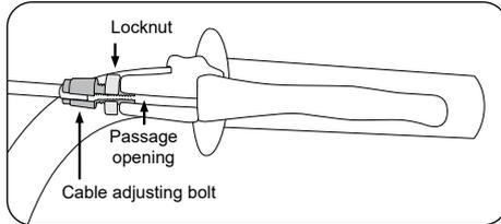
2. Push the arms of the front wheel brake together with your hand. Clip the cable fitting onto the brake lever. The cable must be passed through the passage opening on the cable adjusting bolt (see the illustration under Point 1).
