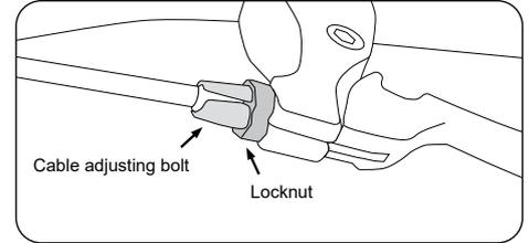
The brake lever can be adjusted to fit different hand sizes. The distance between the lever and the handlebars can be adjusted.
