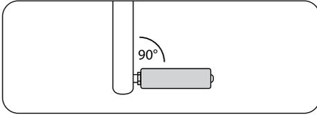
Apply assembly grease to both threads before assembling the pedals.
