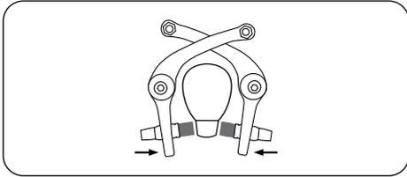
2. Loosen the bolt or nut on the cable clamp (by turning it anti-clockwise) until the cable can be moved.
