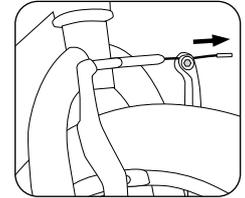
4. Tighten the cable clamp. The torque is **7-8Nm**
