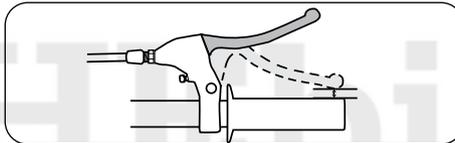
1. Squeeze the brake to check the free travel of the lever and the bite point.
